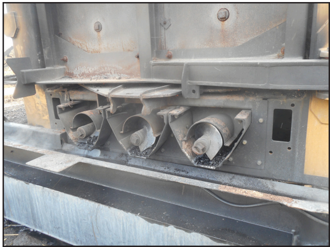
Augers push out steaming biochar, which resembles the crunchy remnants of a quenched campfire. Steve McLaughlin photo.
