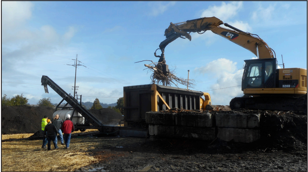
The Carbonator 6050 is a moveable unit that converts 20 tons of wood waste and slash per hour into 1,800 pounds of agriculture-friendly biochar, sequestering about a quarter of the total carbon. Steve McLaughlin photo.
